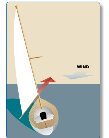
Fig 10 Helmsman's eye view. The boom points the way to go when turning into the wind.
