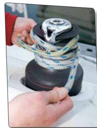
Fig 5 An extra turn or two after the self-tailing section secures the sheet and is quick to remove.
